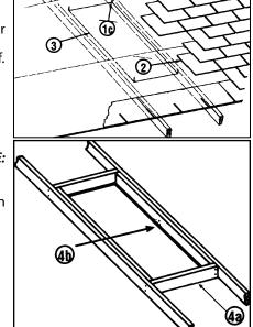
Flash curb (sizes 2525, 2549, 3333, 3349, 4949 can be used with Sun-Tek's preformed, pre-cut Step Flash Kit with one-piece head and sill). Use galvanized sheet metal, aluminum, or copper. Metal should extend a minimum of 4" over shingles (on bottom side), then up sides of curb. Flashing should be flush with curb top. 1283.IC2 - 9/16 Shingle up sides and across the top.
