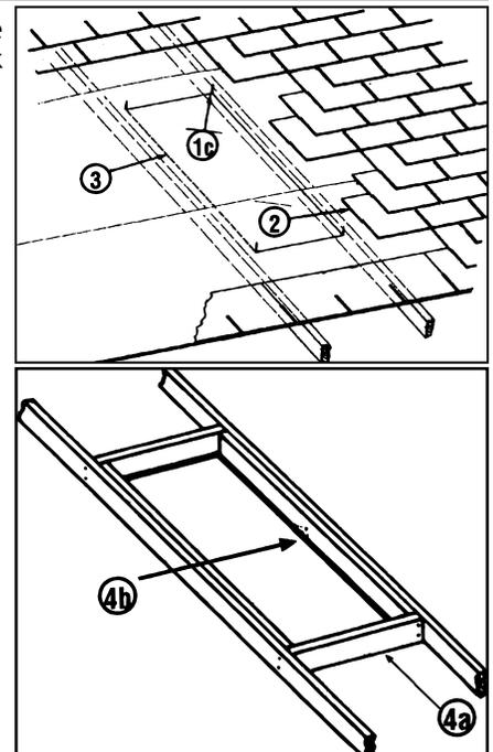
**IMPORTANT: Bottom flange of skylight MUST go on top of shingles.**
