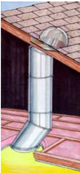
The 10 inch diameter Sun-Tek Tube sells for about $150 and brings light to small spaces.
