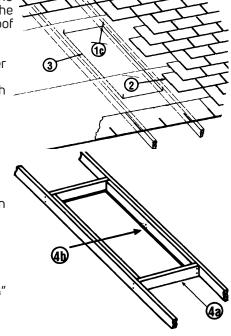
IMPORTANT: Bottom flange of skylight MUST go on top of shingles.
